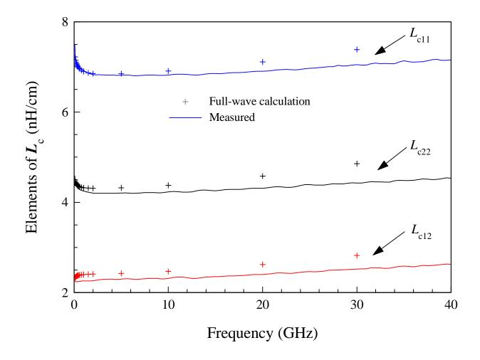
Figure 3. The elements of  $L_c$ . Solid lines refer to measurements while markers indicate values from the full-wave calculation method of [13].c:\htb386\coupled\asym\plots\l.plt
