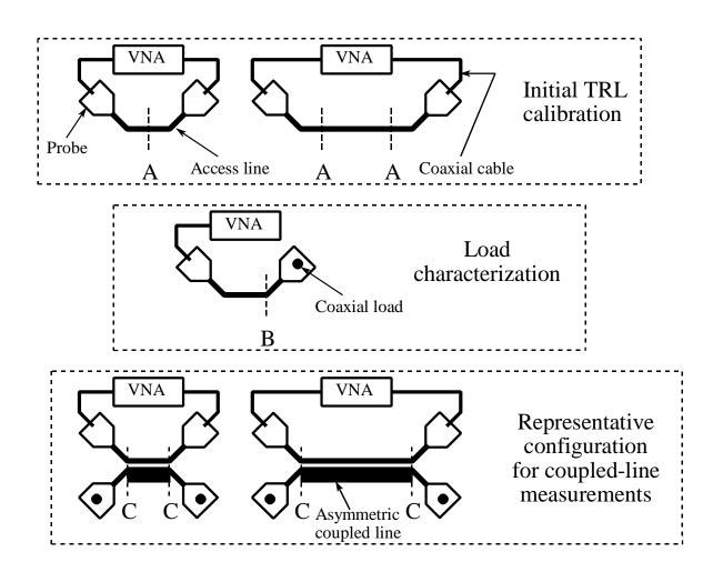
Figure 2. A schematic representation of the measurement artifacts and procedure. Coaxial cables connect the vector network analyzer (VNA) to the ground-signal-ground probes. The probes contact the center conductor of the access lines directly; the ground contact is made with metallized via-holes. c:\dr\coupled\multimod\fig1.wpg
