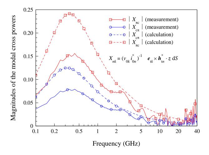
Figure 5. The measured magnitudes of the off-diagonal elements of the modal cross-power matrix *X*. Solid lines refer to measurements, dashed lines refer to values from the full-wave calculation method of [13]. c:\htb386\coupled\asym\plots\x.plt
