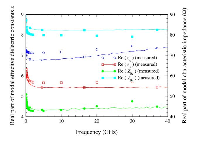
Figure 4. The real part of the measured effective dielectric constants and characteristic impedances of the c and  $\pi$  modes. Solid lines with markers refer to measurements. Markers with no lines indicate values from the full-wave calculation method of [13]. c:\htb386\coupled\asym\plots\all.plt
