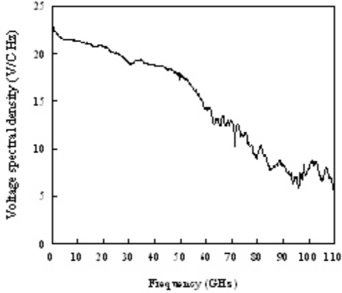
Figure 1. Representative measurement of a check-standard voltage spectral density.
