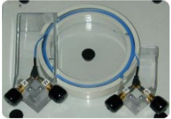
A differential transmission line; one of the multiport test devices.
