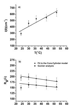
**Figure 3.** Results of the Guinier analysis of the SANS data of the block copolymers in 2.0 wt.%  $D_2O$ . Key: (a) I(0) as a function of temperature; (b)  $R_g$  as a function of temperature. The radius of the core of the micelles has a polydispersity of 0.15 based on the modeling of the SANS data, which defined the error bars of the  $R_g$  shown in the figure. The solid lines in Figure 3 are guides to the eye.
