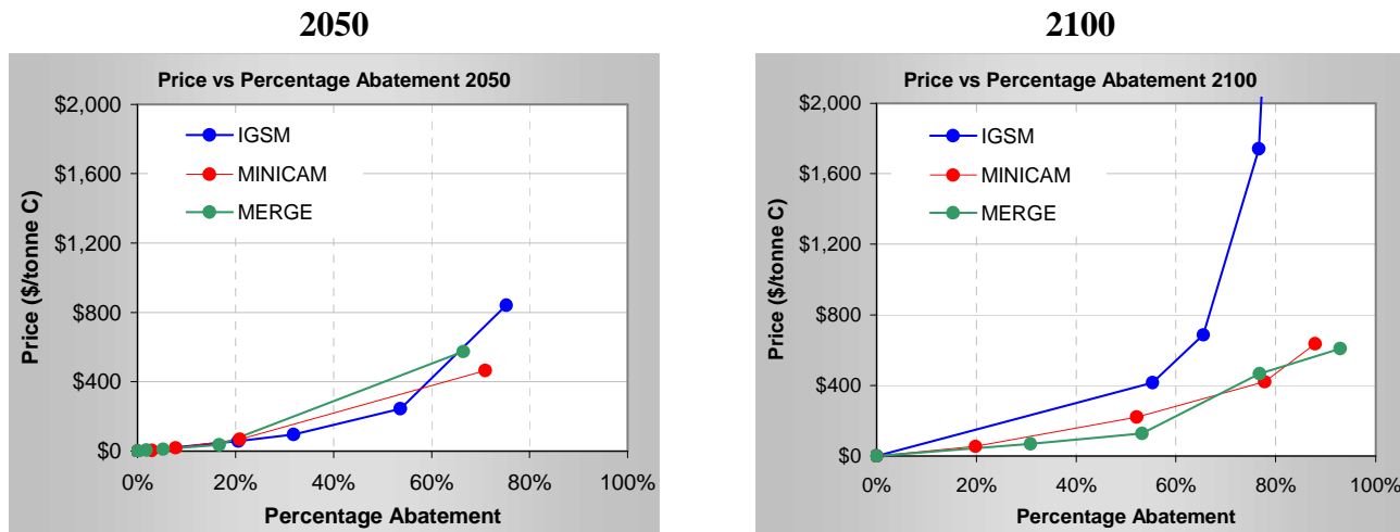
Figure ES.13. Relationship Between Carbon Price and Percentage Abatement in 2050 and 2100: The relationship between carbon price and percentage abatement is very similar among the models in 2050. In 2100, the relationship between carbon price and abatement diverges across the models, due in large part to different assumptions regarding the technologies available to facilitate emissions reductions late in the century. (Note that CO 2 emissions vary across the reference scenarios from the three modeling groups, so that similar percentage reductions, as shown in this figure, imply differing levels of total emissions reduction.)
