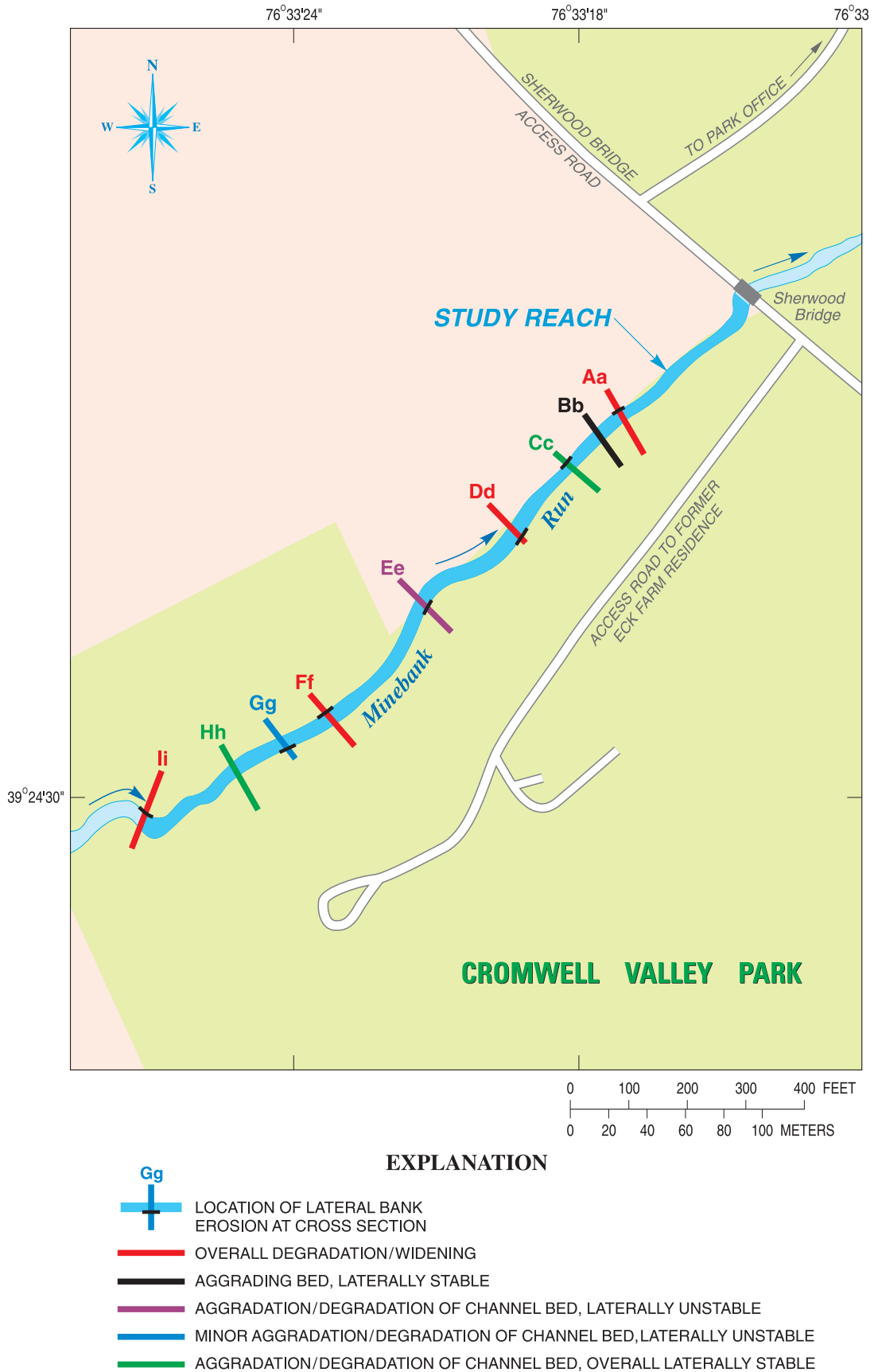
Figure 27. Summary of pre-restoration geomorphic conditions in the Minebank Run study reach, 2002 through 2004.
