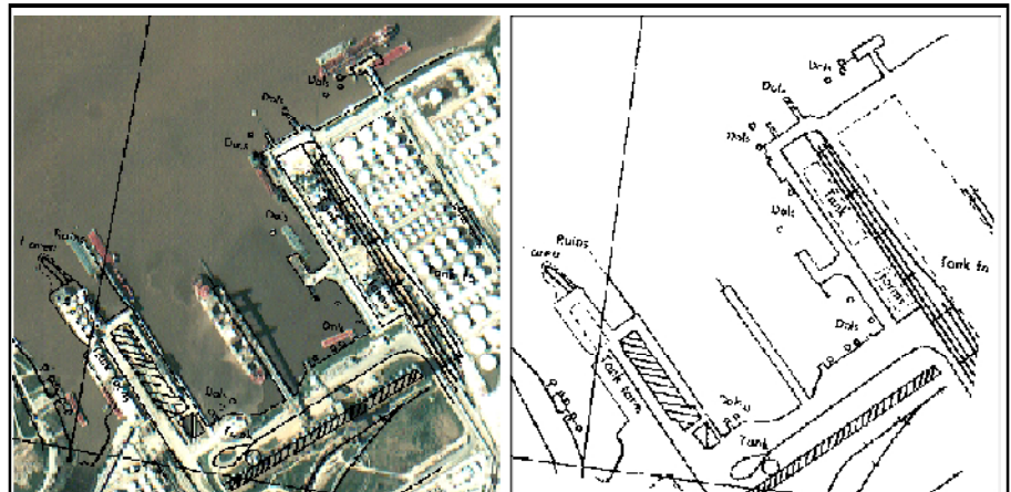
Example of NOAA's shoreline mapping activity for New Orleans, Louisiana. The image on the left is an aerial photograph. The image on right displays the shoreline derived from the photograph that is used on NOAA's nautical charts. Stereo photogrammetry with tide-coordinated, GPS-positioned aerial photography is used by NOAA to accurately delineate the shoreline.
