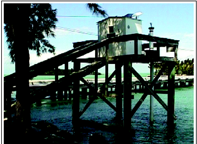
The NOAA tide station at Vaca Key, Florida Bay, supplies water level and storm surge data, wind speed, and air and water temperature to the community. This station is part of NOAA's National Water Level Observation Network (NWLON) comprised of 175 stations around the U.S. coast, including the Great Lakes and ocean island possessions and territories. Station data are transmitted ever 6 minutes to NOAA and made available over the Web to the public.
