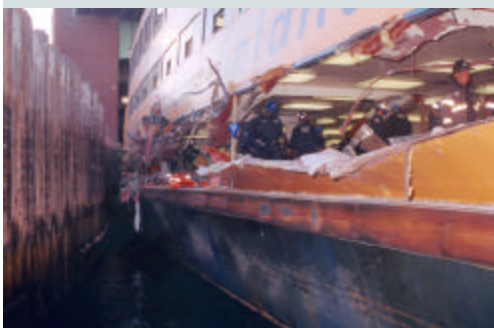
Damage to the ferry Andrew J. Barberi .
