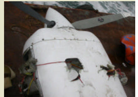
The right engine of the Air Sunshine Cessna 402c, which ditched in the waters off of the Bahamas.
