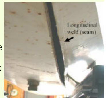
The failed seam on a nurse tank in Calamus, Iowa
