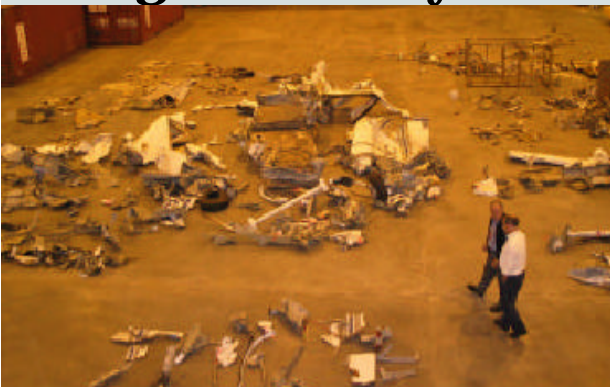
Investigators examine the wreckage of a Cessna 208 cargo plane at the NTSB Academy's laboratory.
