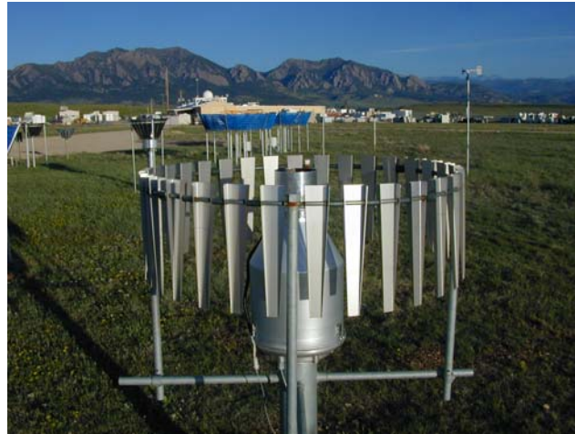
Figure 3-1. Single Alter Wind Shield Type
