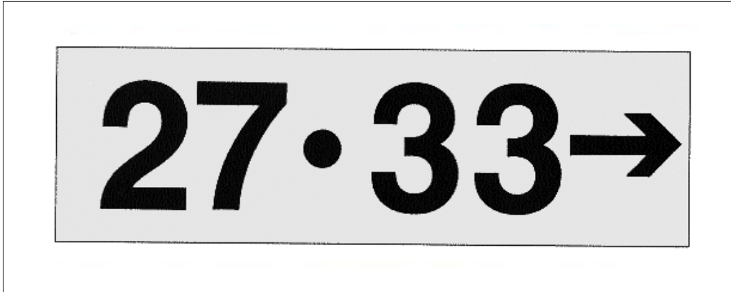
FIG AD 1.1-48 Destination Sign for Common Taxiing Route to Two Runways
