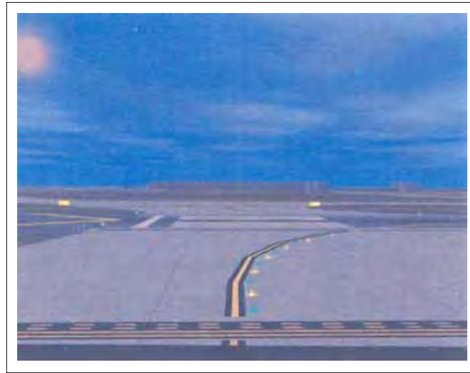
FIG AD 1.1-9 Taxiway Lead-On Light Configuration
