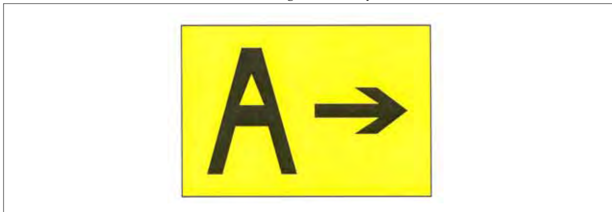
FIG AD 1.1-45 Direction Sign for Runway Exit
