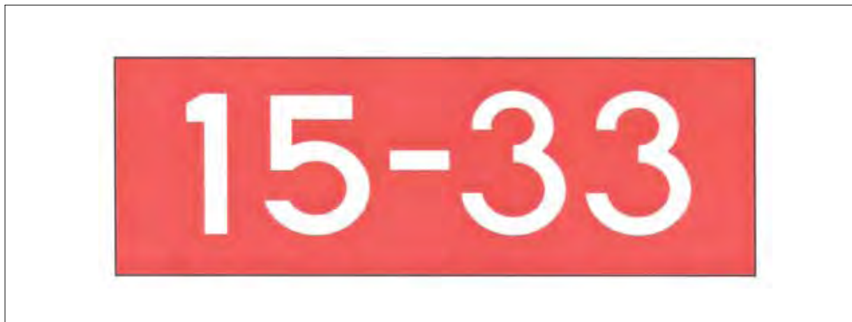
FIG AD 1.1-33 Runway Holding Position Sign
