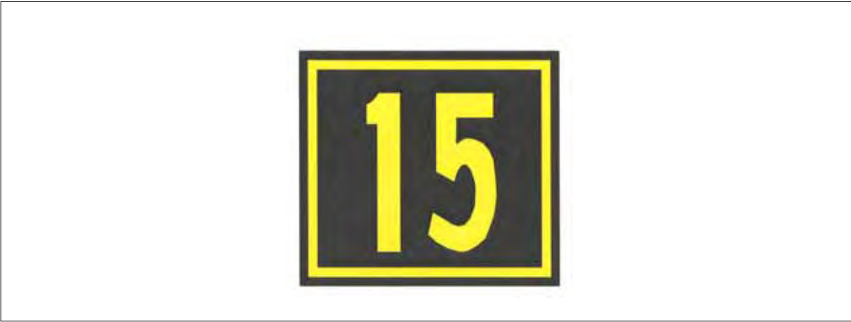
FIG AD 1.1-41 Runway Location Sign
