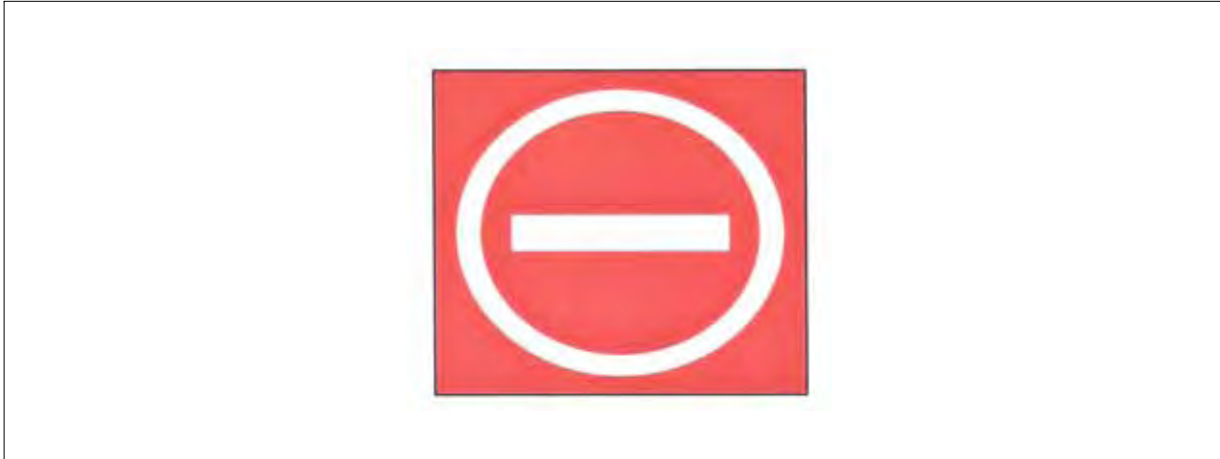
FIG AD 1.1-38 Sign Prohibiting Aircraft Entry into an Area
