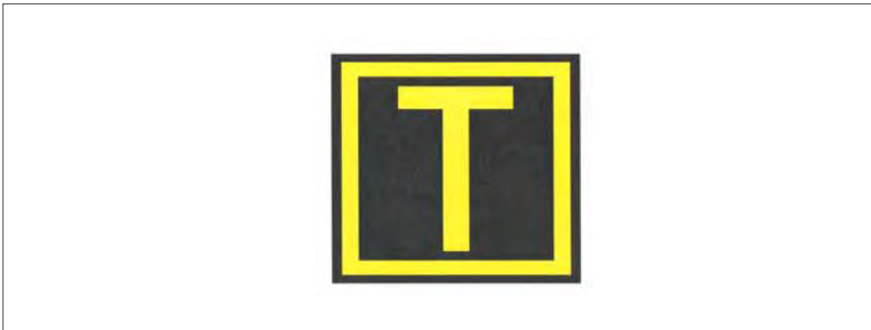
FIG AD 1.1-39 Taxiway Location Sign
