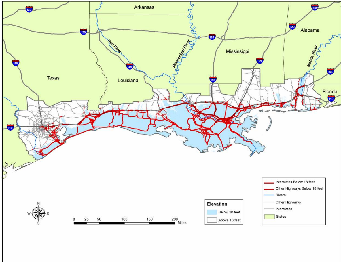
Figure 4.5 Highways at risk from storm surge at elevations currently below 5.5 m (18 ft). (Source: Cambridge Systematics analysis of U.S. DOT data)
