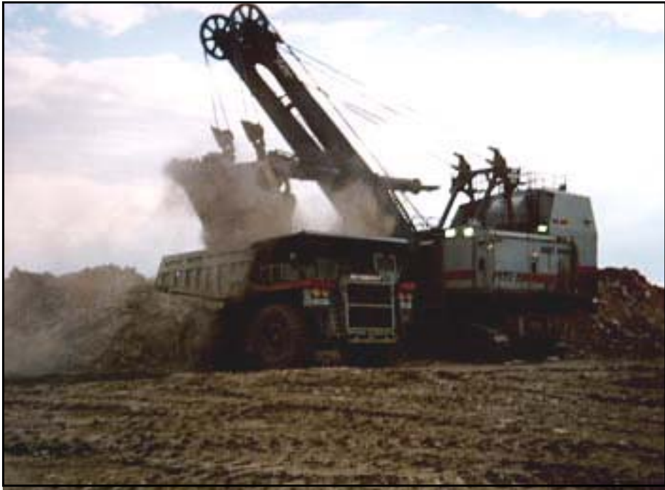
Figure 1-1. A MTM operation in West Virginia. The purpose of these operations are to remove mountaintops in order to make the underlying coal accessible.
