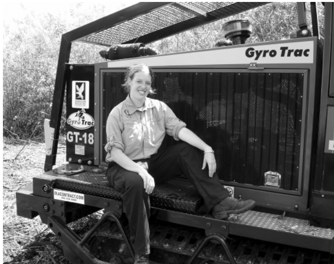
Intern Jenn D'Emilio at Big Cypress National Preserve in Florida with the GyroTrac, a machine used for mechanical fuels reduction
