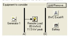
On the schematic, notice the arrow that now connects the load button to the AC bus and shows the direction of energy flow. Also note that the label you typed, "Remote Load," appears on the schematic, along with the values of the average and peak demand.
