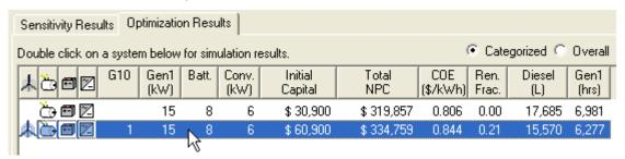
In the Simulation Results window, you can view many technical and economic details about each system configuration that HOMER simulates. For this example, click the Electrical tab, and note that 16% of the total electric energy produced by the system is excess electricity, or energy that is not used by the system and goes to waste. Would including more batteries in the system design result in this excess electricity being used by the system?
