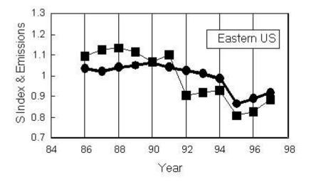
Changes in sulfur air quality east of the Mississippi and national changes in emissions of sulfur from all sources (solid line) and from electric utility point sources alone (dashed line). The air quality indices are averages of the air chemistry and precipitation chemistry results.
