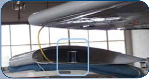
A multifilter radiometer is positioned inside the Cessna's new starboard wingtip extension.
