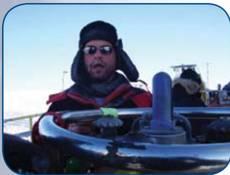
Dr. Dave Turner, co-leader of the field campaign, works on a dewar containing liquid helium, a cryogenic liquid required by the TAFTS instrument to cool its detectors. This greatly improves the signal-to-noise ratio of the observations.
