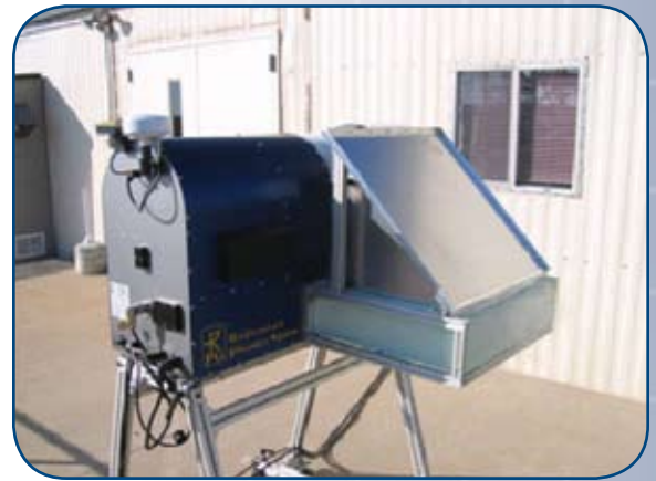
The triangular container on the right contains liquid nitrogen needed for initial calibration of the new high-frequency (90/150 GHz) microwave radiometer.
