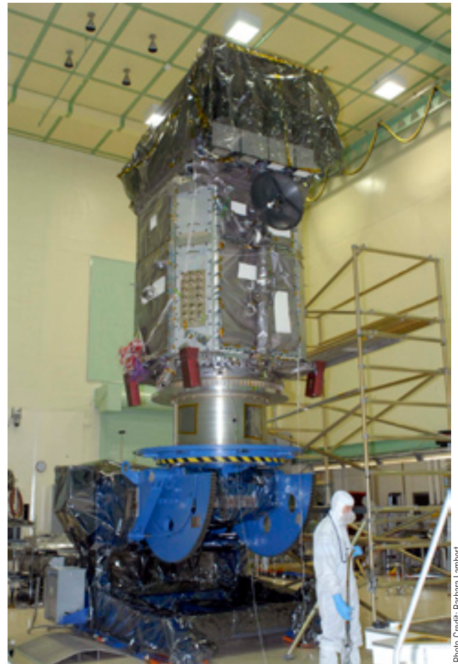
Caption: SDO undergoes a second round of comprehensive performance testing (CPT #2) following dynamic testing that included vibrations, shocks, and acoustics.
