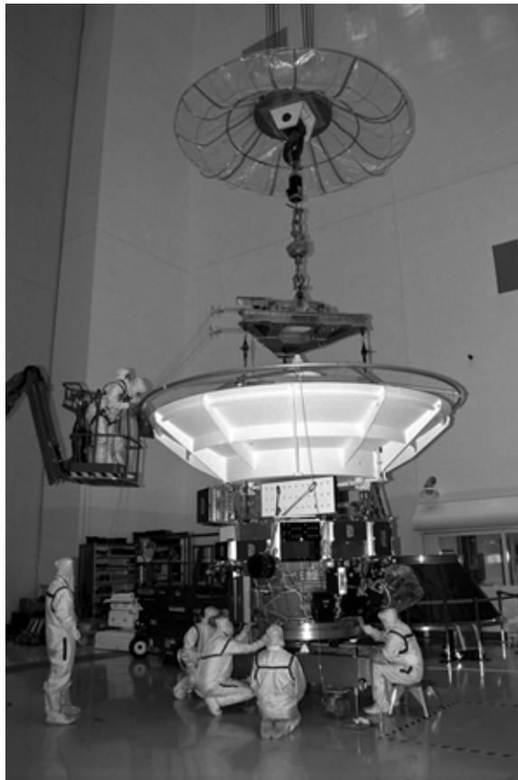
Most spacecraft are safe on their dolly: workers separate Cassini's upper equipment module from its dolly.
