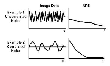
Figure 3, Schematic of the NPS (one-dimensionally) representing the noise attributes of a digital radiographic system.
