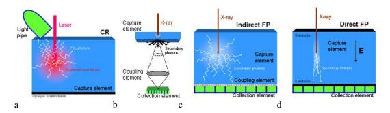
Figure 1. Conceptual schematic of detector components in CR (a), CCD-based (b), indirect flat-panel (c) and direct flat-panel (d) systems (Used by permission from 4. Samei E. Performance of Digital Radiography Detectors: Factors Affecting Sharpness and Noise. In: Advances in Digital Radiography, E Samei (ed). Radiological Society of North America (RSNA) Publication, Categorical Course Syllabus, Oak Brook, IL, 2003, pp. 49-61).
