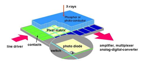
Figure 3. Schematic of a flat-panel detector.
