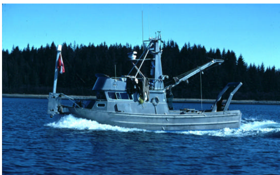
The tracking vessel with bow-mounted retractable rotating dual hydrophone.
