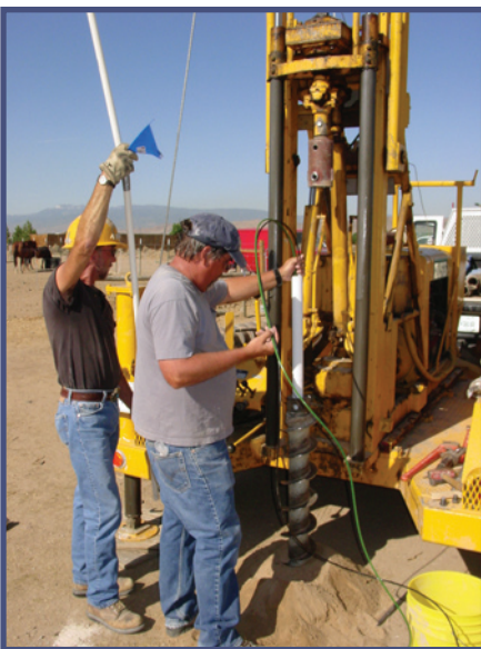
Placing a suction-cup lysimeter, sealing the hole with bentonite, and final hole showing sampling line after being backfilled with native soil. Left and center photographs by Christian Kropf; right photograph by Michael R. Rosen.
