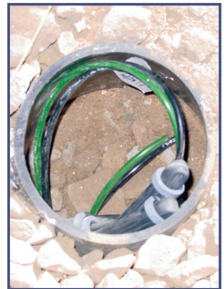
Placing a suction-cup lysimeter, sealing the hole with bentonite, and final hole showing sampling line after being backfilled with native soil. Left and center photographs by Christian Kropf; right photograph by Michael R. Rosen.
