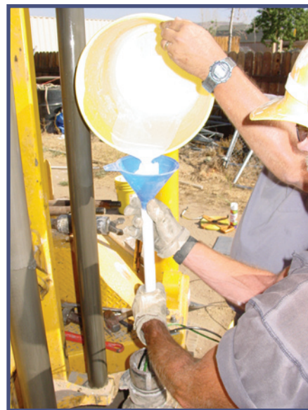
Placing a suction-cup lysimeter, sealing the hole with bentonite, and final hole showing sampling line after being backfilled with native soil. Left and center photographs by Christian Kropf; right photograph by Michael R. Rosen.
