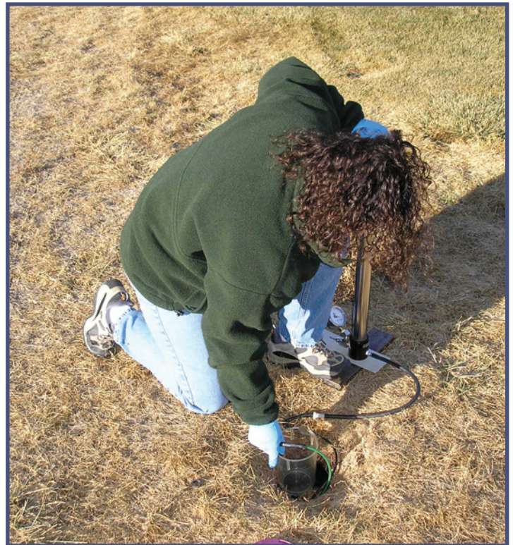
Retrieving soil water sample from suction-cup lysimeter. Photograph by Anna Makowski, University of Nevada, Reno.
