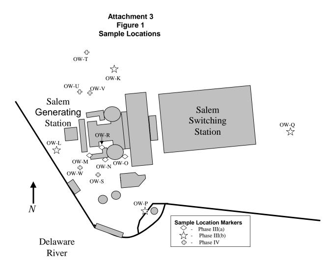
Figure 1 depicts observation well (OW) sample locations for ground water sampling. See Table 1 for results. Locations R, M, N, O are located inside the coffer dam. (Figure provided by PSEG)
