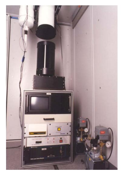
The MPL works just like the Ceilometer but can see clouds that are much higher. The MPL can detect cirrus clouds in the tropics, which can be as high as 16-17 kilometers above the ground.
