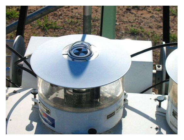
The Black & White PSP measures the amount of solar radiation (sunshine) that falls on the sensor under the clear dome.
