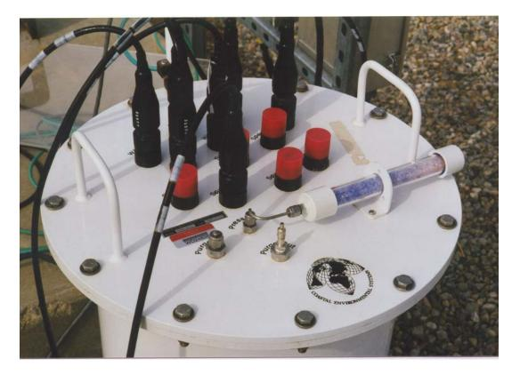
A barometer is housed inside the white cylinder at the base of the meteorological tower. A tube connects the barometer to the outside. Moisture is prevented from entering the barometer by a larger tube filled with water absorbing material. This cylinder also contains a special type of computer (called a datalogger) that collects from the instruments.
