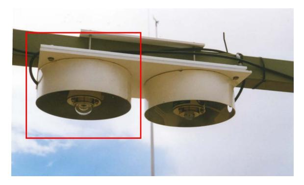
The PSP measures the amount of solar radiation (sunshine) that falls on the sensor under the clear dome.
