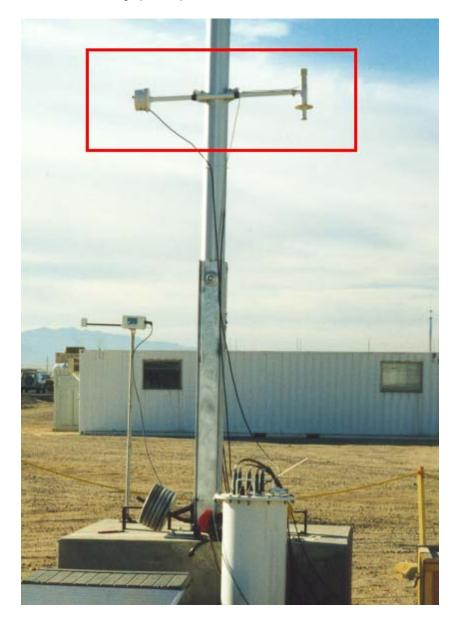
The temperature and humidity sensors are mounted inside a tube to protect them from direct sunlight. The tube is attached to the meteorological tower near the bottom. A small fan at one end draws air into the tube and over the sensors.
