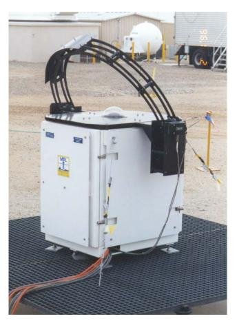
The Whole Sky Imager (WSI) is an automated imager used for assessing and documenting cloud fields and cloud field dynamics. The WSI is a ground-based electronic imaging system that monitors the upper hemisphere. It captures sky images. We can then assess the presence, distribution, shape, and radiance of clouds over the entire sky using automated cloud decision algorithms and related processing.
