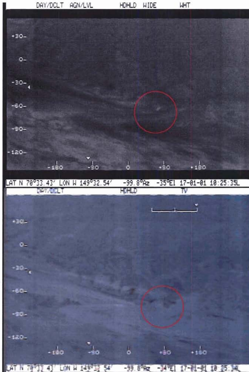
Figure 17a: Use a combination of video and FLIR to help weed out suspicious hot spots. The top image shows what appears to be a promising hot spot. The bottom image indicates the spot is merely the exposed soil of an eroding bank. The spot is also very high on the bank.
