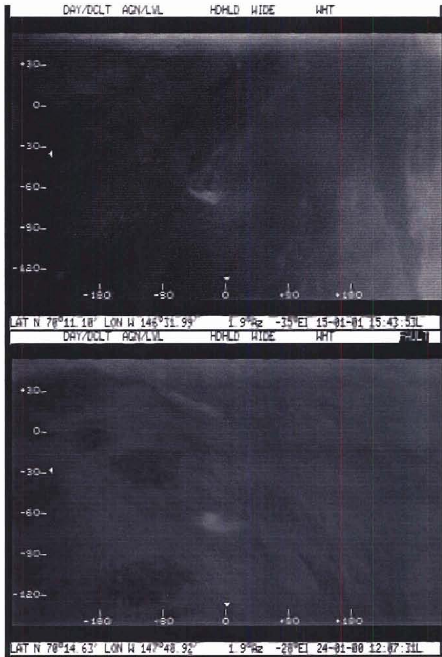
Figure 10: Two images of known dens in the narrow field of view mode of FLIR (zoom). The shape of the heat signature in the lower image actually reflected the internal geometry of the den structure.
