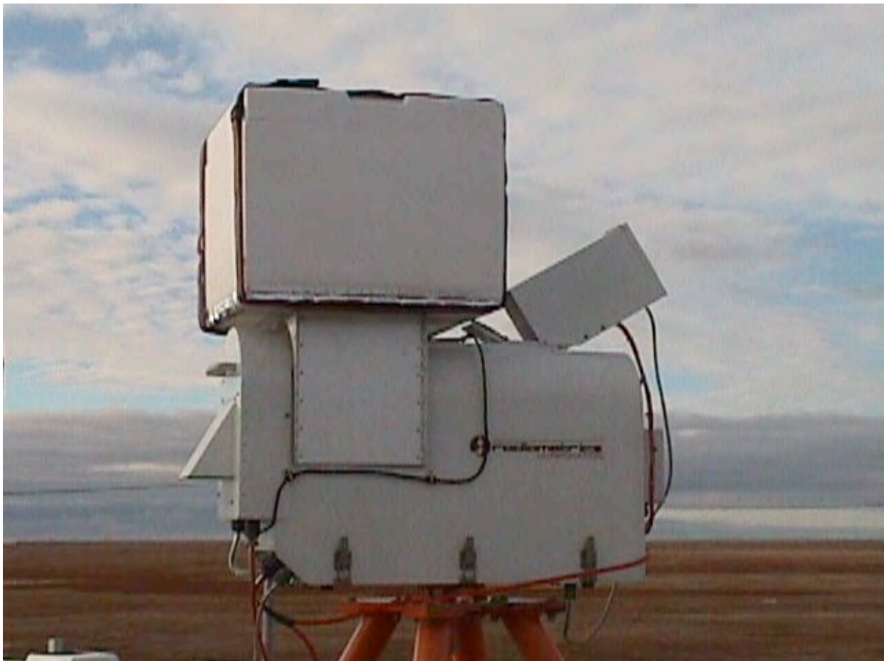
Figure 9. The Microwave Radiometer Profiler (MWRP) at Barrow, Alaska with the LN 2 -filled Styrofoam target in place during calibration of the V-band channels in September 2000.
