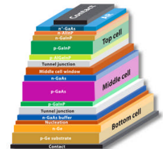
A multi-layered triple-junction solar cell designed to absorb different solar photons.
