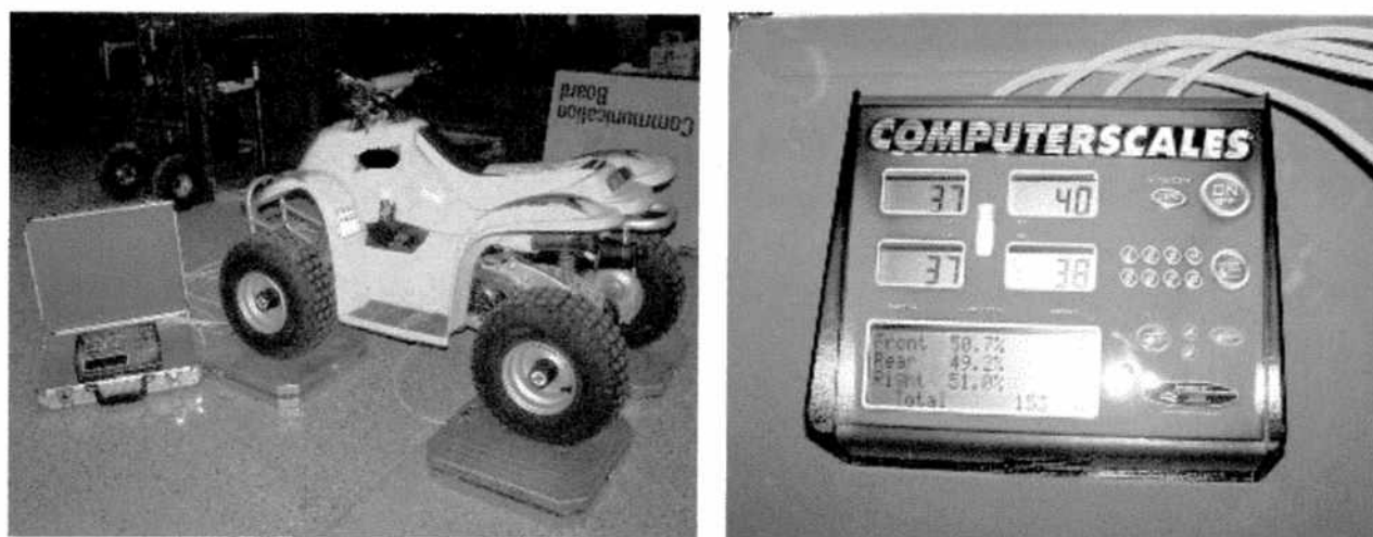
Figure 1. ATV Weight Measurement on Wheel Scales
