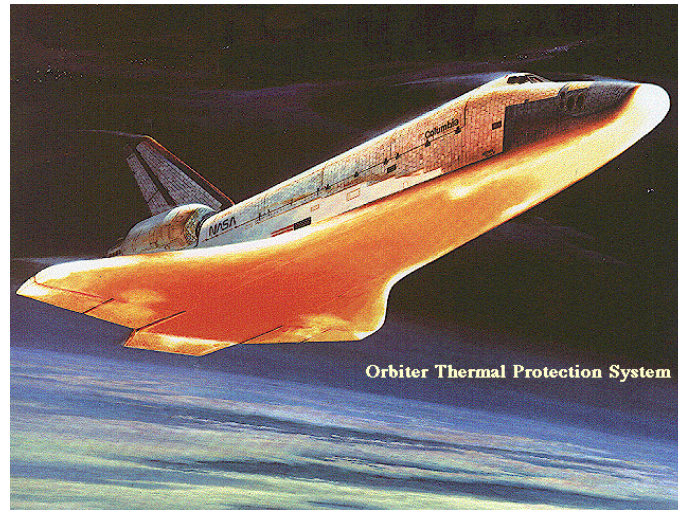
Figure 15. Drawing of Space Shuttle Orbiter during reentry conditions. (Drawing reprinted courtesy of NASA).
