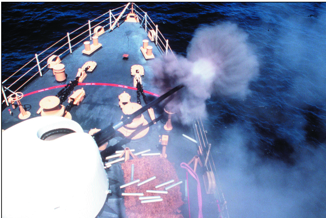
A Bear-class medium endurance cutter fires its 76-mm/62-caliber gun during live-fire exercises.
