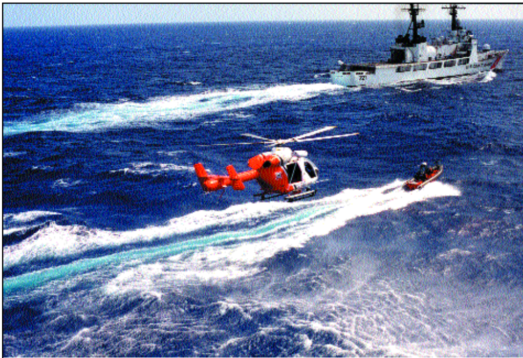
The high-endurance cutter Gallatin (WHEC 721) operates with a proof-of-concept MH-90 Enforcer helicopter and an Over-the-Horizon Rigid Hull Inflatable Boat (OTH RHIB), both of which were specifically designed to engage “go-fast” drug smuggling boats.
