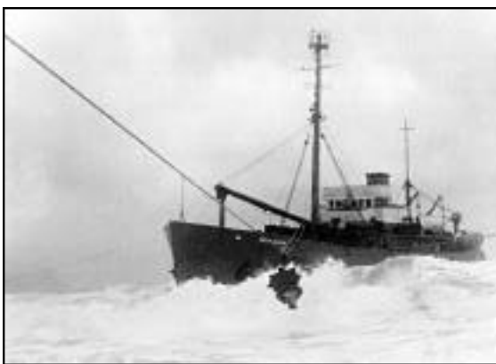
A crewmember from a ship run aground is rescued via breeches buoy during a violent storm.
