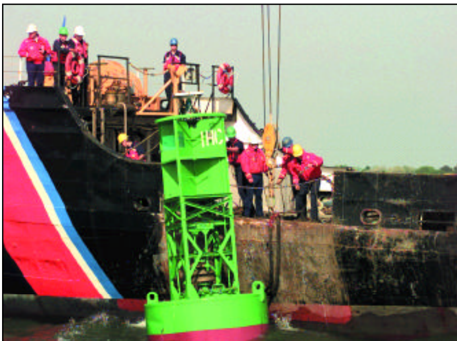
The crew of the cutter Hornbeam (WLB 394) prepares to lift a buoy out of the water off Yorktown, Virginia.
