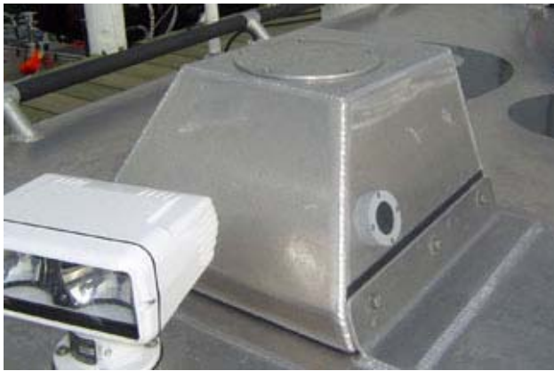
Figure 3-52 Thermal Imaging Camera Mounting Platform
