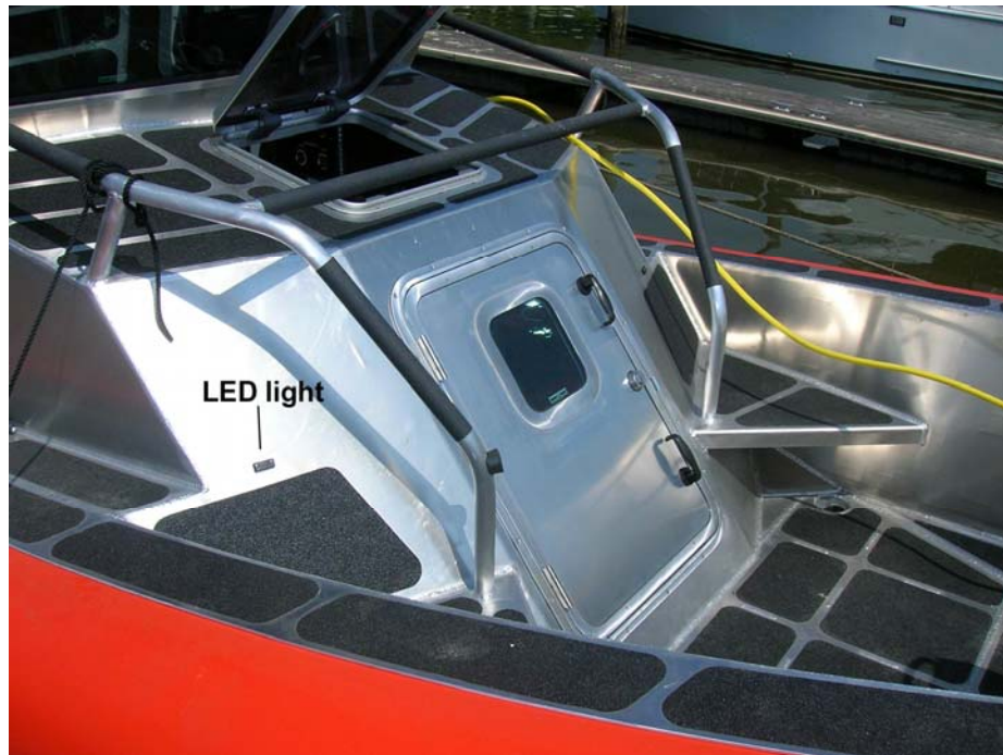
Figure 2-25 Forward Weather Deck LED
