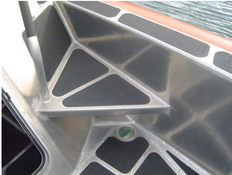
Figure 3-26 Forward Weather Deck Drains
