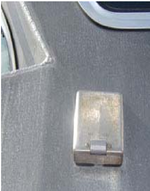
Figure 3-67 Shore Power Connection
