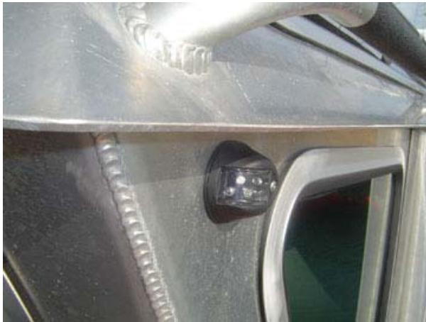
Figure 3-82 Port Navigation Light
