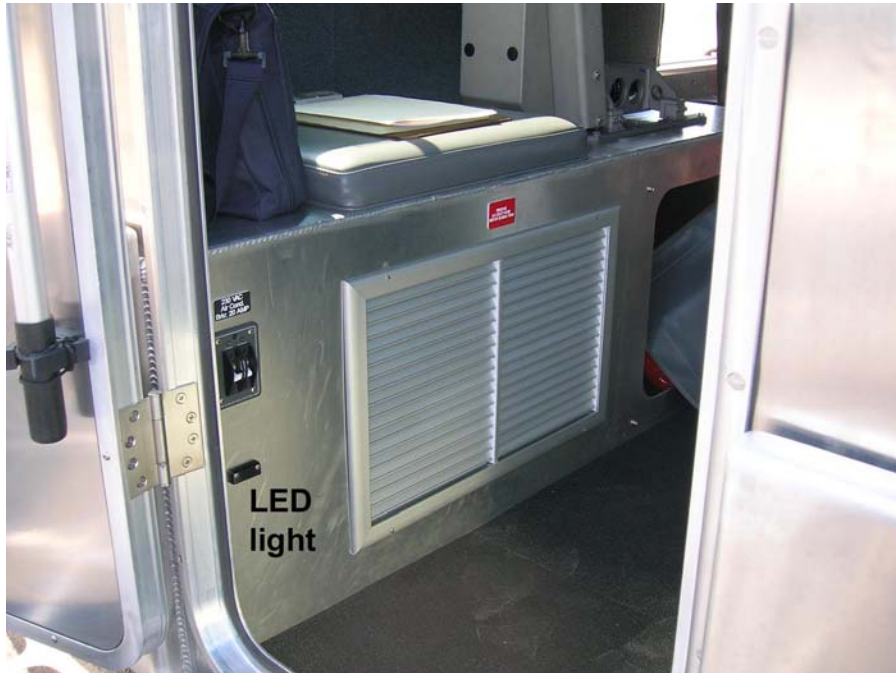
Figure 3-86 Interior (Deck Edge) Light
