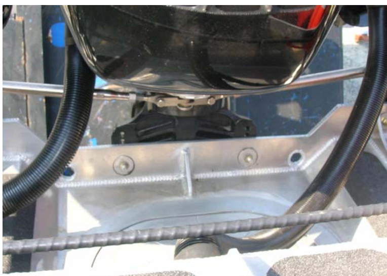
Figure 3-30 Engine Well Drains
