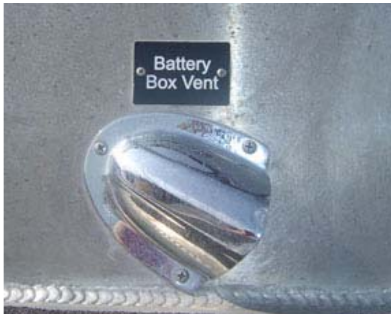
Figure 3-56 Battery Box Vent
