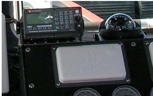
Figure 3-49 Automatic Identification System Transponder
