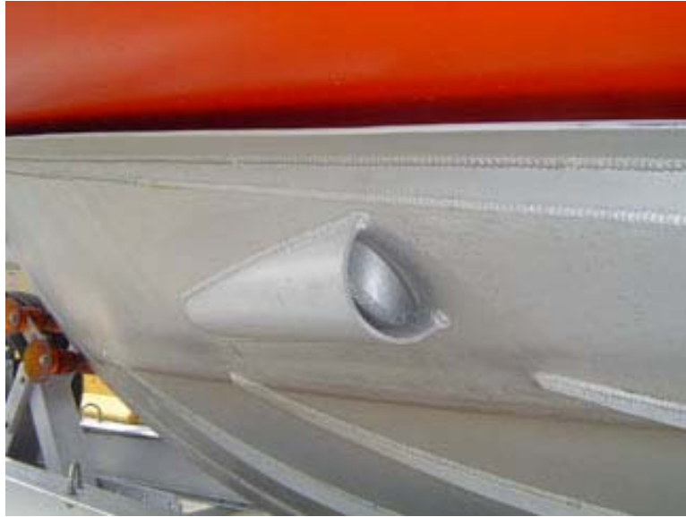
Figure 3-27 Forward Weather Deck Scupper
