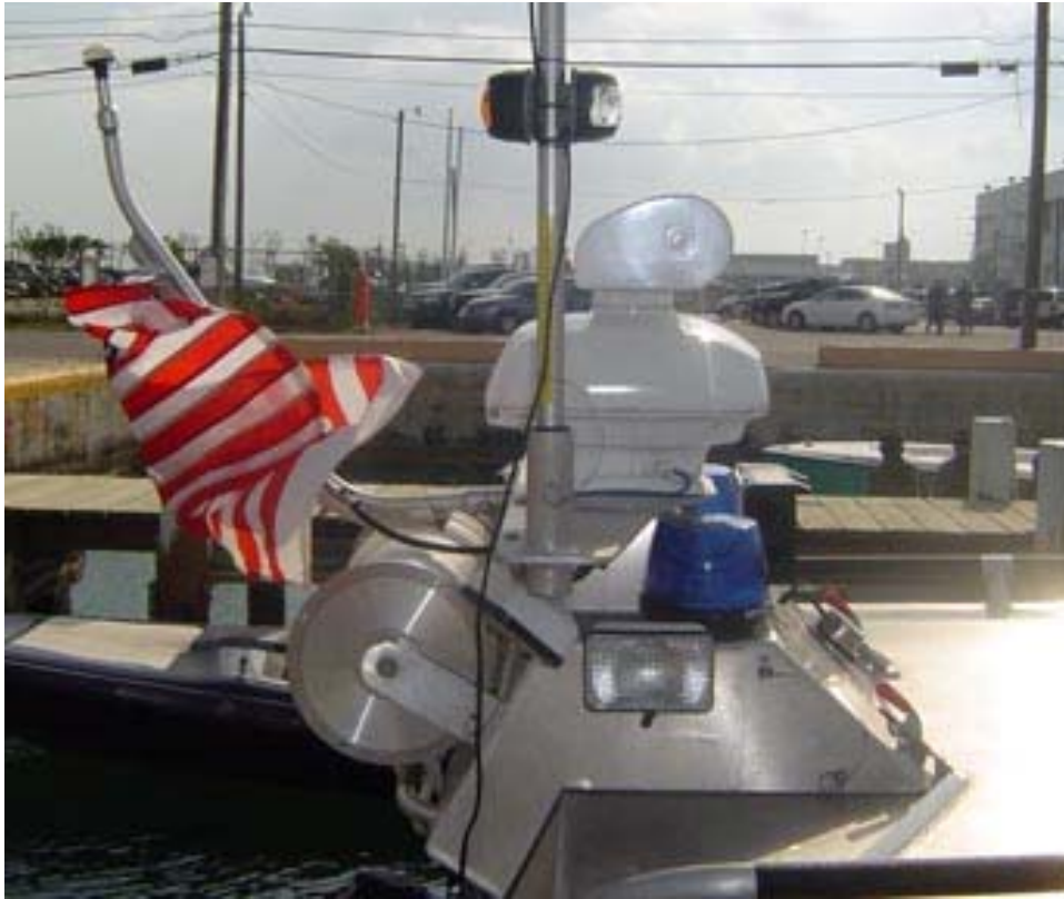
Figure 3-84 Anchor/Masthead Light, Floodlights, Strobe Lights
