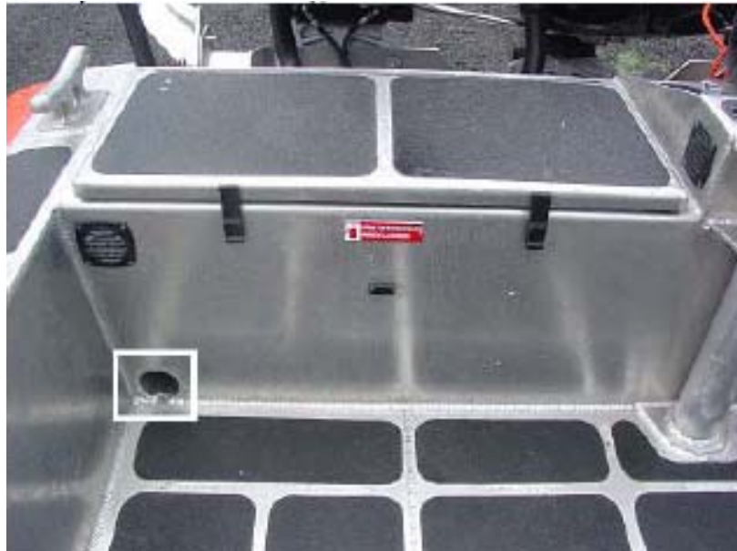
Figure 3-28 Aft Weather Deck Drain
