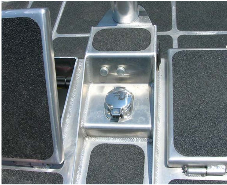
Figure 3-36 Fuel Tank Fill
