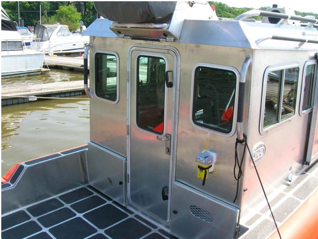
Figure 2-9 Aft Cabin Windows and Weather-Tight Door
