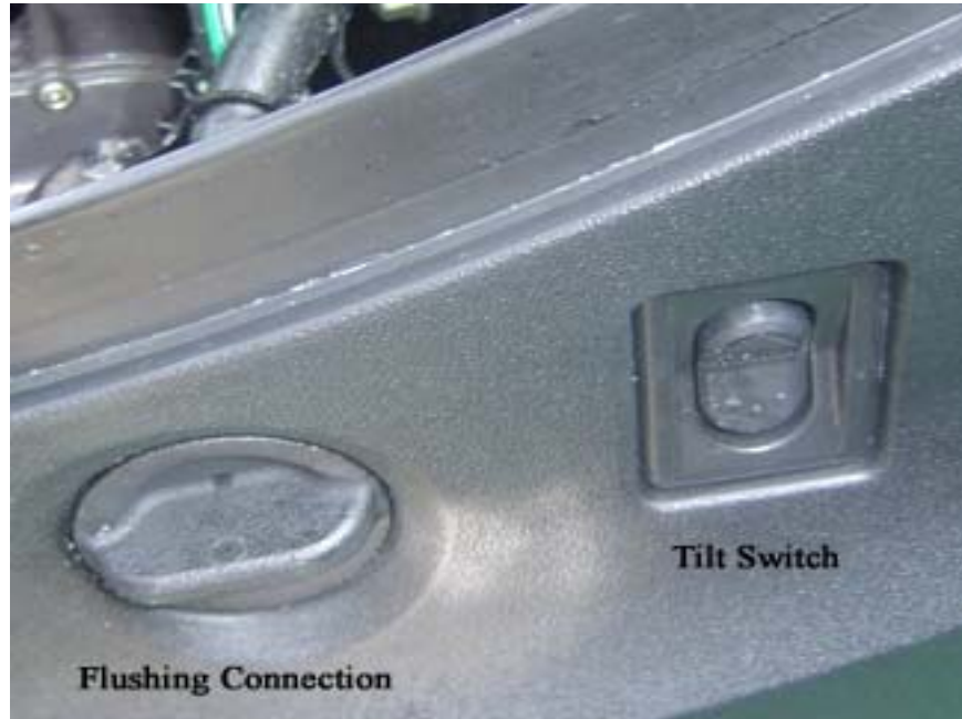
Figure 3-16 Power Tilt Switch and Flushing Connection
