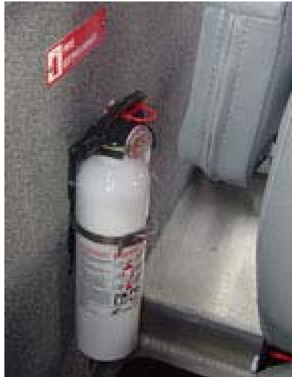
Figure 3-92 B-1 Type Fire Extinguisher
