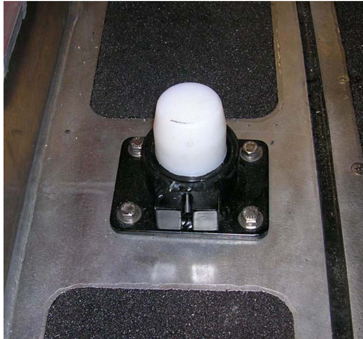
Figure 2-9 Antenna Arch Deck Fitting
