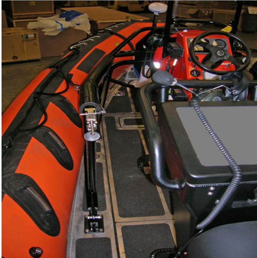
Figure 2-8 Antenna arch (Lowered on Foredeck)
