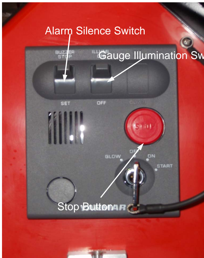
Figure 3-10 Start/Stop and Alarm Annunciator Panel
