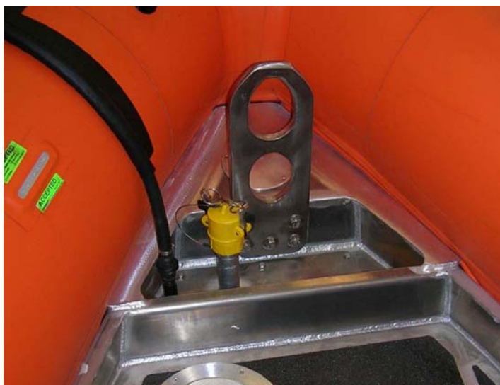
Figure 3-18 Fuel Fill Station
