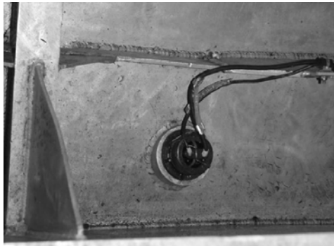
Figure 3-28 235DT-SSE Depth and Temperature Sensor
