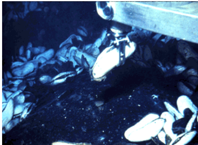
The manipulator arm of the research submersible Alvin collecting a giant clam from the deep ocean floor. (Photograph by John M. Edmond, Massachusetts Institute of Technology.)
