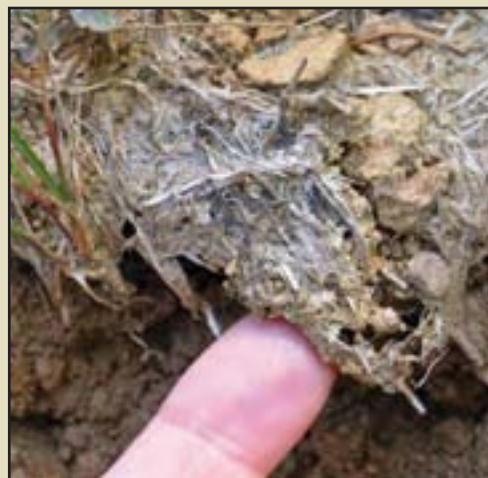
Figure 10.105 – Hydraulic mulch with tackifiers remain effective for up to a year. This hydraulic mulch and tackifier slurry was applied nine months prior to this picture, and was still partially effective.
