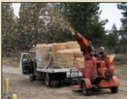
Figure 10.23 – Straw blowers range in size from machines which can apply 30 to 60 bales per hour (shown here) to very large straw blowers that can shoot up to 20 tons per hour.
