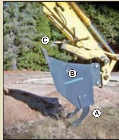
Figure 10.10 – The subsoiling grapple rake is a quick-mounting attachment to excavating machinery that combines several operations in one: (A) subsoiling with winged tines, (B) soil incorporation with bucket, and (C) removal of rock and slash with grapples (Photo courtesy of Mike Karr, Umpqua National Forest).
