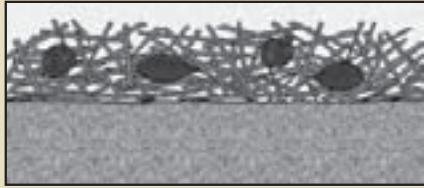
Figure 10.94 – Seeds mixed into long-fibered mulch have less contact with soil, which can reduce germination.
