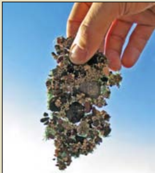
Figure 10.103 – Hydraulic mulch applied at high rates and with specialized tackifiers will hold together as a sheet and is referred to as a “bonded fiber matrix,” or BFM. The application rate of wood fiber mulch in this picture was 3,000 lb/ac.
