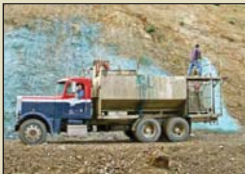
Figure 10.97 – The hydraulic seeder is composed of a tank that holds and mixes a slurry, and a pump system that moves the slurry through a nozzle for application to the soil surface.
