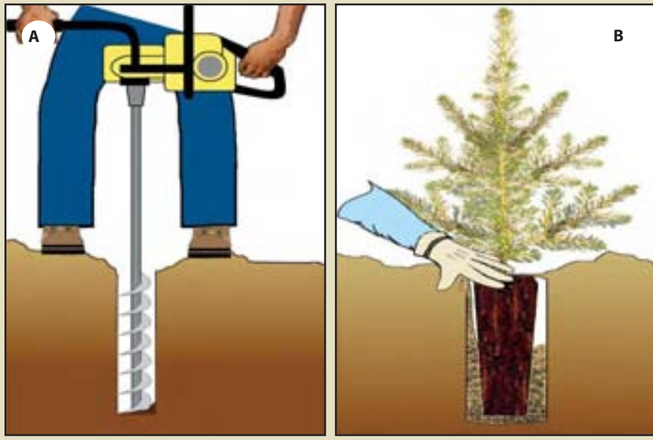
Figure 10.121 – Power augers are effective because one trained operator determines the depth and spacing of the planting holes (A). Auger bits come in a variety of sizes to accommodate the large stocktypes favored in restoration plantings (B).
