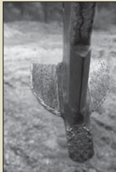
Figure 10.8 – Soil shattering becomes more effective when wings are mounted on subsoil tines. This equipment is called a winged subsoiler. Photo courtesy Brent Roath.
