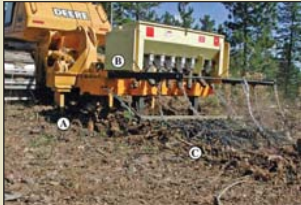
Figure 10.90 – The “ripper-seeder-harrow” equipment was developed by the Umatilla National Forest. This equipment prepares the soil surface and mixes the seeds into the surface in one
