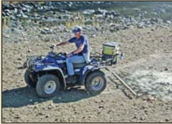
Figure 10.91 – Seed sowing and mixing equipment can be attached to most types of ground based equipment, including all-terrain vehicles. A seed spreader attached to the back of an all-terrain vehicle broadcasts seeds on the soil surface and a chain harrow mixes seeds into the soil.
