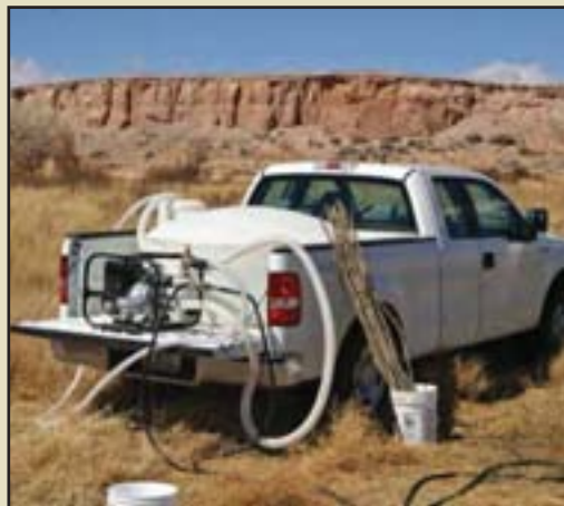
Figure 10.111 – A 250-gallon water tank with pump can be installed in the bed of a pickup truck to supply water for Waterjet Stinger sticking.
