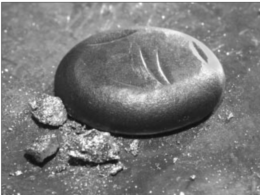
The yttrium-silver button shows dents and deformation from repeated hammer blows. The gadolinium-silicon-germanium material was shattered with a light tap from the hammer.
