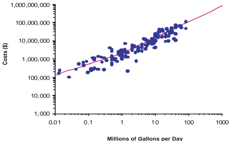
The investment need for each system in the sample was estimated based on the reported and modeled costs of each project in the sample. The total need for medium and large systems was then estimated for each state by applying the sample weights to the total need for each system. The need for each system was multiplied by the sample weights; this product was then summed across all systems to produce the total need for medium and large systems in each state.
