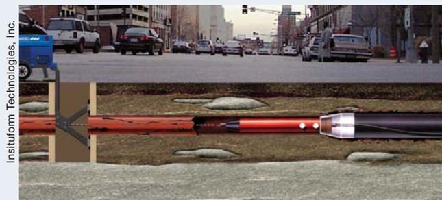
*Pipebursting is an effective way to upgrade deteriorated pipe. A pneumatic bursting head is attached to new pipe and threaded through the old pipe. As it passes through the old pipe, the bursting head destroys the old pipe, compacting it into the surrounding soil—making room for the new pipe of the same or even larger diameter. Pipebursting is a preferred method of pipe upgrade since it is semi-trenchless and minimizes disruption to streets, homes, and businesses in the area.*
