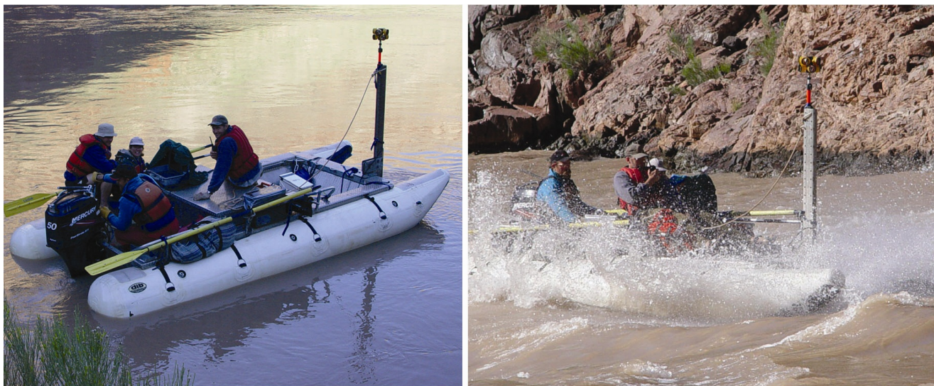
Figure 2. Photos of operation of ADV boat in quiet water above the rapid (left) and within the wave field of the rapid (right). (Photos: C. Watkins)
