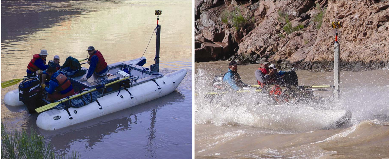
Figure 4.2: Photos of operation of ADV boat (left) in quiet water above the rapid and (right) within the wave field of the rapid (photographs by C. Watkins).
