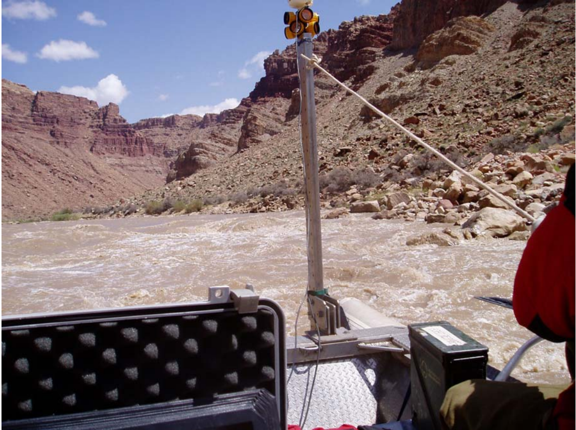
Figure 5.4: View of the front of the boat in Rapid 13 of Cataract Canyon while the ADCP is deployed. The 360° prism and the bottom of the GPS receiver are shown mounted to the top of the boom assembly (photograph by T. Kenney).
