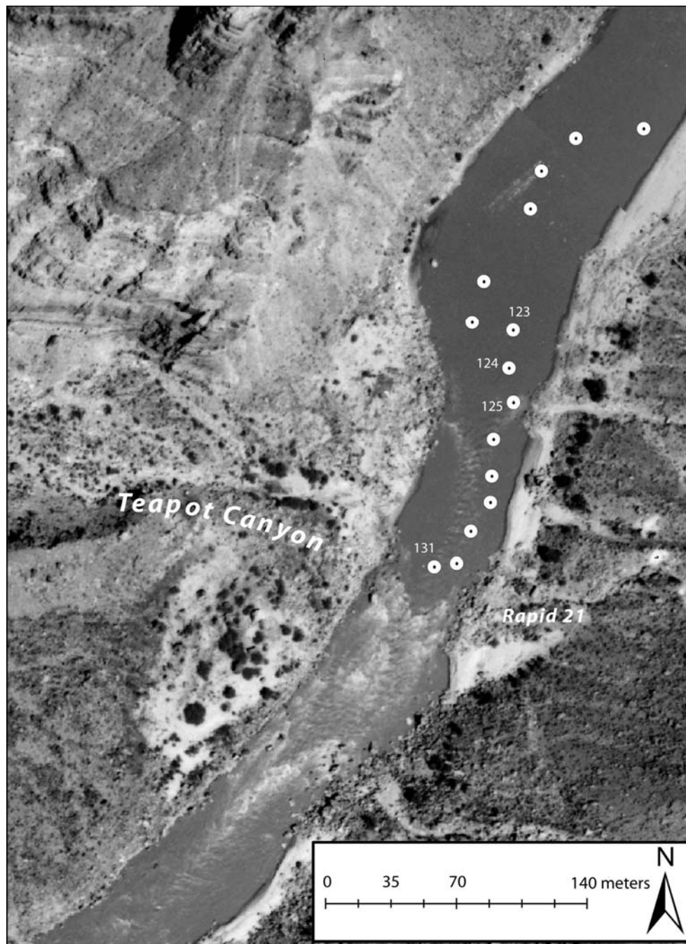
Figure 5.6: Locations of velocity measurements made in Cataract Canyon at Rapid 21. Rapid 21, also known as Big Drop 1, is one of the larger rapids in Cataract Canyon. Rapid 20 (not shown) is 500 m upstream of Rapid 21 and influences the flow in the pool above Big Drop 1. Flow is from top to bottom. Numbers refer to specific survey-point locations referenced in the text.
