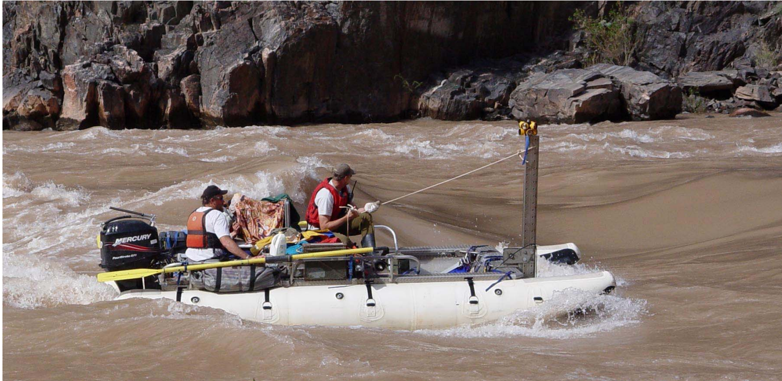
Figure 5.1: Boat equipped to make flow velocity measurements in Salt Creek Rapid within Grand Canyon. Diane Boyer is under the sun shade monitoring the computer and making field notes (photograph by C. Watkins).
