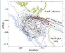
Composite of eddy outlines from 95 cloudfree turbidity maps over 7 years of satellite data; eddy generally follows isobaths (blue) and has a diameter of approximately 50 km. Figure courtesy of K.Edwards, Univ. of Washington. Turbidity derived from NASA SeaWiFS data by R.Stumpf, NOAA.
