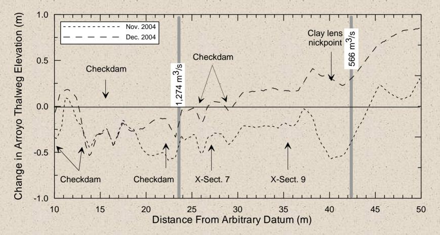
Changes in thalweg elevation are with reference to a common datum defined by the 1996 pre-flood elevation; data above the horizontal solid line at 0.0 indicate deposition, data below indicate erosion.
