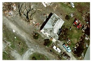
**Typical F0 Tornado Damage**Note the trees are stripped of leaves, but the trees remain standing. Only light roof damage and a few missing shingles.
