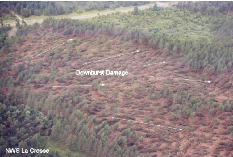
Figure 4: The tree damage in this photo was a result of an intense downburst. Notice the divergent damage pattern caused by the spreading out of winds. In contrast, tornadoes produce convergent damage signatures.
