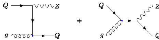
Fig. 4.15. Leading order Feynman diagrams for producing a Z-boson in association with a heavy quark, Q, at hadron-hadron colliders.
