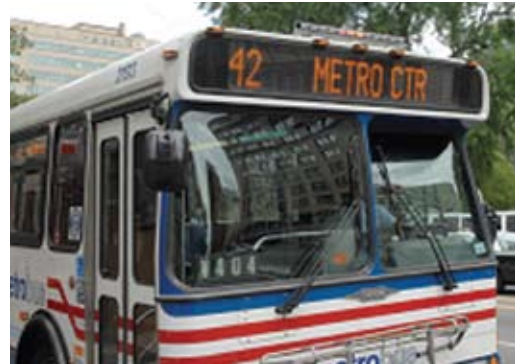
Safety innovations, such as the strobe lights shown above the destination display on this WMATA bus, can increase the visibility of buses and improve the safety of pedestrians as they access transit.
