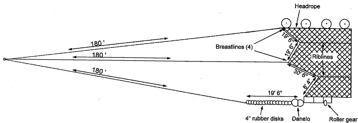
Figure A-1.--Schematic diagram of the 90-105 polyethylene Nor'easterly bottom trawl, roller gear and accessory gear used during the 1993 Gulf of Alaska triennial bottom trawl survey.
